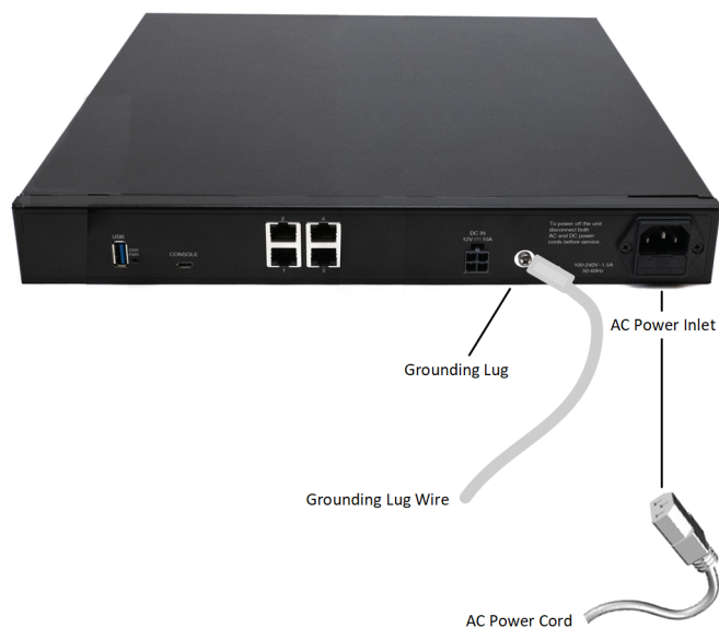
Figure 5-1: Connecting AudioCodes Mediant 800C device to the power
